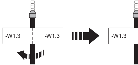
Figure 4-7 Example of a cable flag
